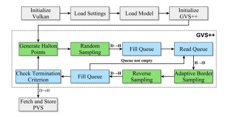
Fig. 5. An overview of the implementation of GVS++. Green boxes represent components that are implemented on the device. Blue boxes are components that are implemented on the host side. The Halton point generation, as well as random sampling, are implemented as separate shaders. The adaptive border and reverse sampling are realized as a single common shader.  $D \rightarrow H$  and  $H \rightarrow D$  show that data is transferred from device to host and vice versa.
