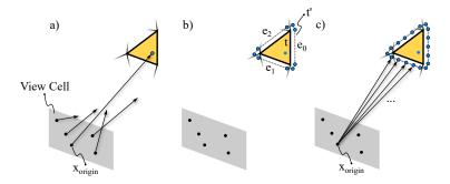
Fig. 2. The adaptive border sampling procedure is shown. Random sampling is used to find initial triangles (seed points) (a). Adaptive border sampling enlarges the boundary of the current triangle t to get a 9-vertices polygon t' (b). Additional samples are placed along the edges  $e_0$ ,  $e_1$  and  $e_2$  of t'. Starting from  $x_{\text{origin}}$ , rays are traced to the nine vertices that form t' and to the samples along the edges  $e_i$  (c).
