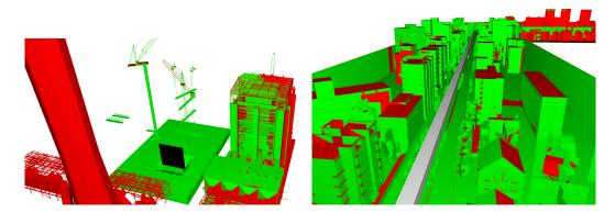
Fig. 1. Triangles that are found to be visible by Guided Visibility Sampling++ (GVS++) are shaded green. GVS++ uses hardware-accelerated ray tracing, achieves low error rates, and is over four orders of magnitude faster than the CPU-based Guided Visibility Sampling implementation. Left: A single rectangular view cell (black region) on the UNC power plant model [UNC 2001]. Right: Multiple rectangular view cells combined to a box-shaped view cell on a city model @VIRES Simulationstechnologie GmbH.
