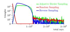
Fig. 10. Detailed plot of the triangles found in one view cell (PPLANT scene, blue in Figure 9) by random sampling (red), adaptive border sampling (blue), and reverse sampling (green) over the number of total traced rays.
